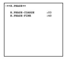
H.Phase adjustment is executed by the HD Controller AK-HRP900.
